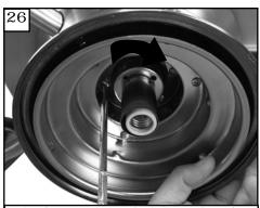
Twist lower cover plate into place by twisting in direction of arrow. Replace 1 screw removed and tighten all 3 screws securely.
